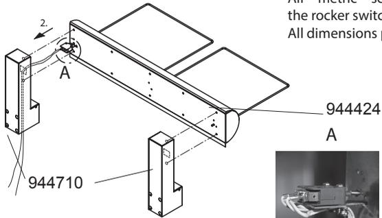
Control cable for rocker switch
