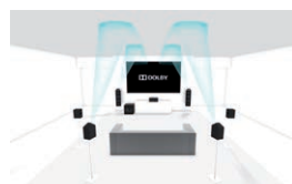
7.1.4: Regular 7.1 setup with 4 ceiling or 4 Dolby Atmos-enabled speakers
