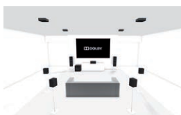
7.1.4: Regular 7.1 setup with 4 ceiling or 4 Dolby Atmos-enabled speakers
