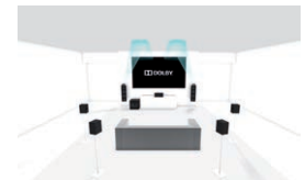
7.1.2: Regular 7.1 setup with 2 ceiling or 2 Dolby Atmos-enabled speakers
