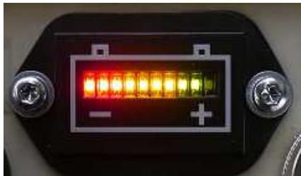
Indication of charge volume of battery system
