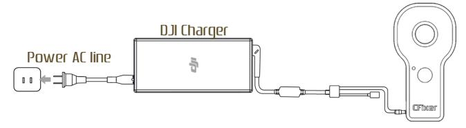
Power supply of the following quadcopters - DJI Phantom 3 Sta / SE, Mavic and Spark – are not designed for CFixer usage. Owners of these multicopters shall use power adapter from their power supply to CFixer (must be purchased separately).
